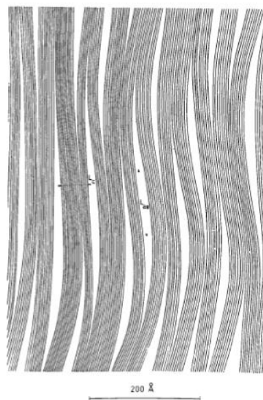
Microstructure of PAN carbon fibers (Orientation of fibers in matrix)
